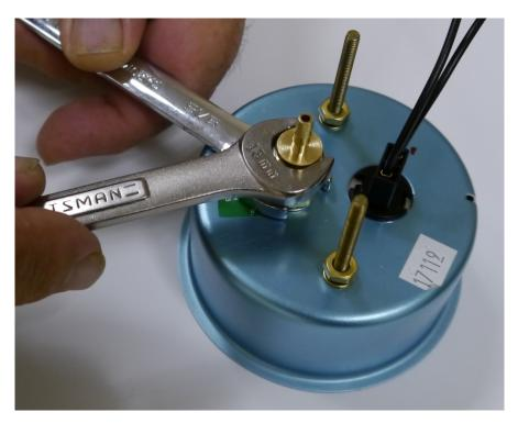
2. Do not over torque the fitting or mounting screws. This will **void the warranty**. See below examples of an over torqued gauge.
